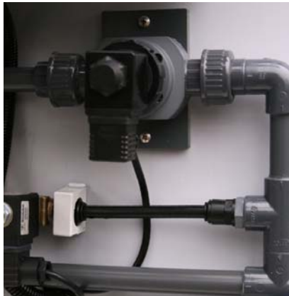
permeate reject valve: rejects the first bad water after starting the R.O. unit; enlarges the capacity of a down stream installed ultra pure water resin
