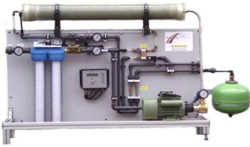
R.O. unit with pressure tank
