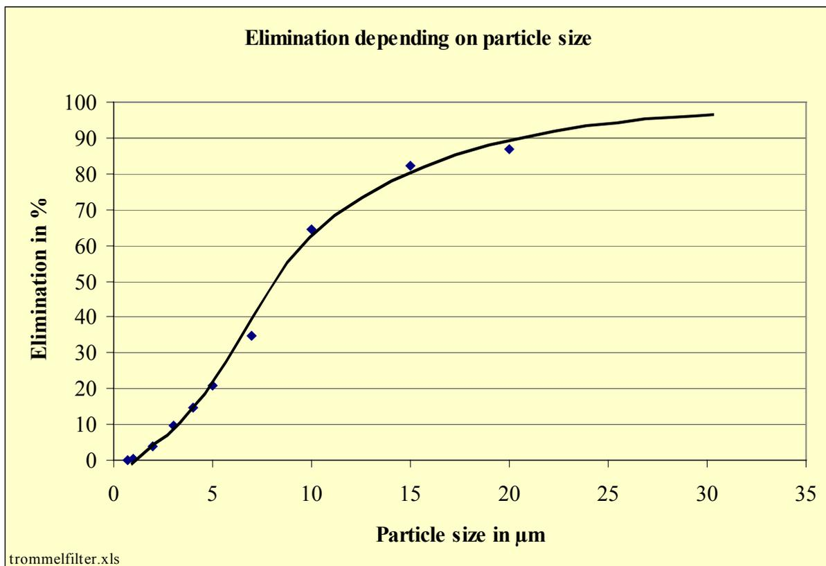
Elimination of particles depending on their size in an AquaCare drum filter with 30 µm sieve.
