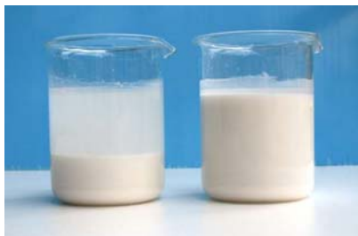
Fresh slurry of limewash ("Kalkmilch"; right) and after about 20 min. time (left): at the bottom the limewash has settled (calcium hydroxide - water - mixture), over it there is the turbid lime water ("Kalkwasser") that you can drop into the aquarium water. Picture: AquaCare
