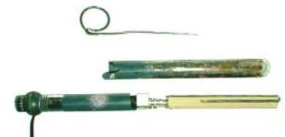
... will overheat. A cracks glass will bring death if a residual-current circuit breaker is not installed. photo: AquaCare
