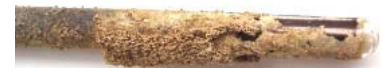
A heater that is not maintained regularly forms lime scale and ... photo: AquaCare
