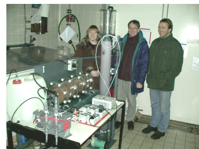
Experimental de-nitrifying system at a temperature of 0°C in the Polar Research Center in Bremerhaven, Germany Image: AquaCare
