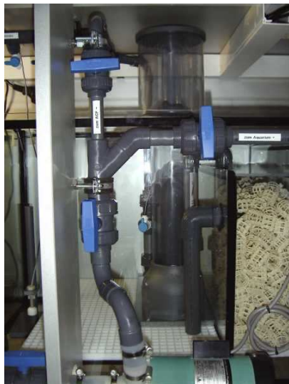
A clearly build tubing made of PVC is a supposition for safe and long-time operation without flooding the living room Image: AquaCare
