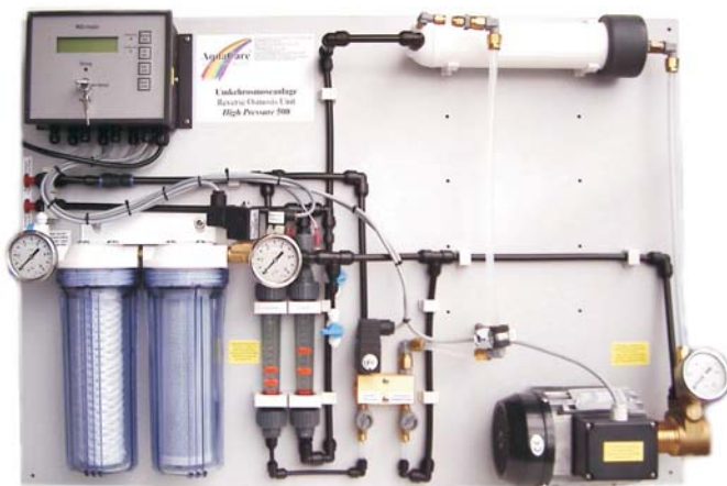
reverse osmosis unit HP 500
