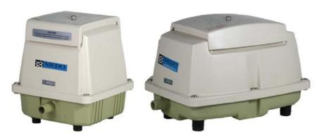
The medo-compressor 1.6...7.2 are very silent units. They are made for heavy duty application. The models 1.6 and 2.7 are equipped with teflon plated aluminium pistons driven with a linear motor. The larger models are equipped with a
