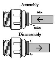
The pressure tube is pushed into the push fit fitting until it cannot be pushed further. The tube should be gently pulled to ensure that the connection is sound. The connection can be released by pushing back the collet and pulling the tube out.
