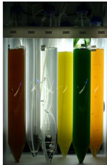
Algae tubes with minimum 4 liters (1 US gal) volume are the minimum for breeding algae for zooplankton picture: AquaCare
