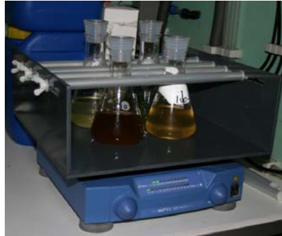
Strain cultures with different algae; here cultivated in Erlenmeyer flasks with sterile plugs on a shaker. picture: AquaCare
