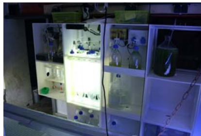
Professional algae breeding unit with some algae tubes (left), algae reactor and the infra-structure picture: AquaCare
