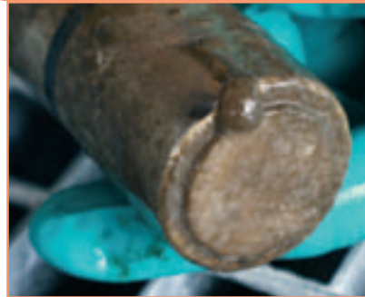
Sensor without ultrasound cleaning system After 16 Days
