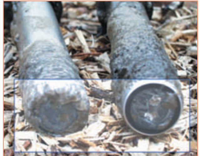
Sensor without and with ultrasound cleaning system after 30 days
