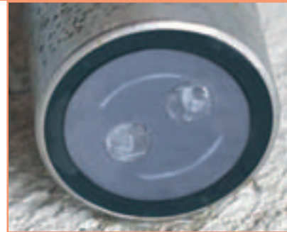
Sensor with ultrasound cleaning system After 16 Days
