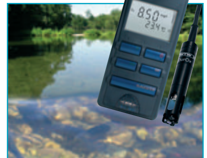
D.O. measurement with Oxi 315i and DurOx® incl. protection cap in fish farming
